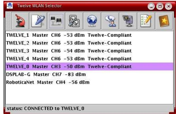
Fig. 6. TWELVE Wireless Selector GUI
