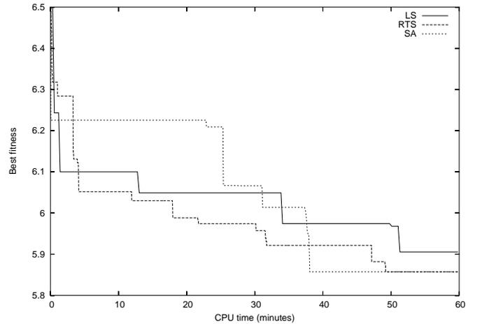
Fig. 5. Localization error —Typical traces for the three algorithms: best solution found against CPU time.
