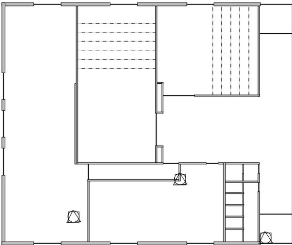
Fig. 9. Localization error —Optimal AP configuration obtained by RTS (triangles), LS (squares) and SA (circles).
