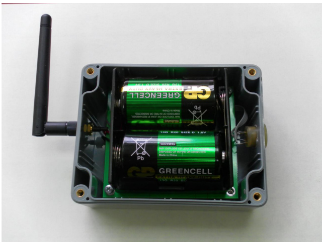
Fig. 3. Wireless gas sensor node in the casing. Visible parts: antenna, power supply (2 × D-batteries, 1.5V), and catalytic sensor (on the right side of packaging).
