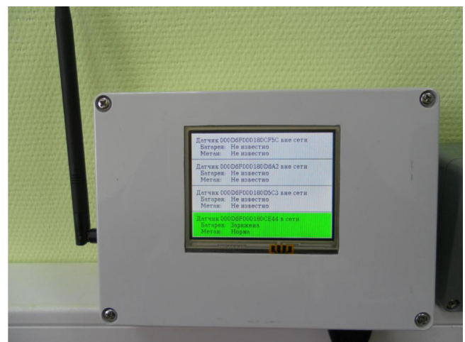
Fig. 5. Network coordinator. LCD display shows the status of the sensor nodes in the network.
