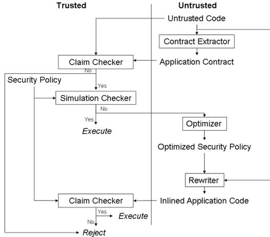
Fig. 4. Optimizer and Rewriter on Untrusted part: Contract Extractor on Untrusted part
