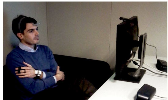
Fig. 1. A viewer, wearing the headphone-like EEG sensor on his head and the watch-like GSR sensor on his left hand while watching the movie.
