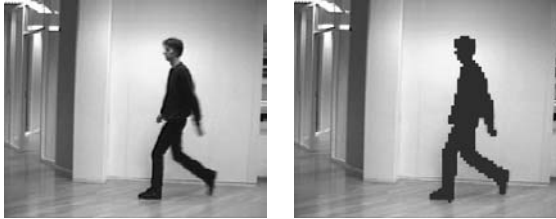
Figure 1. Frame from sequence (left); Segmented blob using background subtraction and Kalman Filtering (right).
