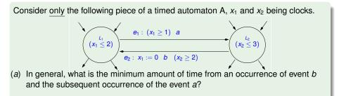
Consider only the following piece of a timed automaton A,  $x_1$  and  $x_2$  being clocks.  $e_1: (x_1 \ge 1)$  a  $e_2: x_1 := 0$  b  $(x_2 \ge 2)$
