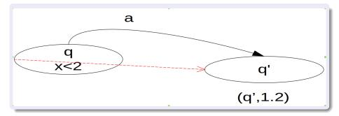
Time Elapse, Switch and their Concatenation •  $\langle q, 0 \rangle \xrightarrow{1.2} \langle q, 1.2 \rangle \xrightarrow{a} \langle q', 1.2 \rangle$  "wait  $\delta$ ; switch;"  $\implies \langle q, 0 \rangle \xrightarrow{1.2+a} \langle q', 1.2 \rangle$  "wait  $\delta$  and switch;"
