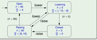
[Solution:  $\Delta t$  is 60 time units. In fact, the maximum value of  $\Delta t$  the controller can afford waiting is given by the minimum time the train may take to reach the gate (70), minus the maximum time taken by the bar to lower, that is, the time taken to lower the angle from 90 to 0 at the lowest absolute speed (90/|-9|). Overall, we have thus  $\Delta t = 70 - 90/(|-9|) = 60$ .]
