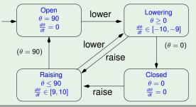
[Solution:  $\Delta t$  is 60 time units. In fact, the maximum value of  $\Delta t$  the controller can afford waiting is given by the minimum time the train may take to reach the gate (70), minus the maximum time taken by the bar to lower, that is, the time taken to lower the angle from 90 to 0 at the lowest absolute speed (90/|-9|). Overall, we have thus  $\Delta t = 70 - 90/(|-9|) = 60$ .]
