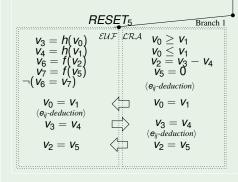
$$\begin{array}{ll} \mathcal{EUF}: & (v_3 = h(v_0)) \land (v_4 = h(v_1)) \land (v_6 = f(v_2)) \land (v_7 = f(v_5)) \land \\ \mathcal{LRA}: & (v_0 \ge v_1) \land (v_0 \le v_1) \land (v_2 = v_3 - v_4) \land (RESET_5 \to (v_5 = 0)) \land \\ Both: & (\neg RESET_5 \to (v_5 = v_8)) \land \neg (v_6 = v_7). \end{array}$$
