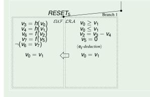
$$\begin{array}{ll} \mathcal{EUF}: & (v_3 = h(v_0)) \land (v_4 = h(v_1)) \land (v_6 = f(v_2)) \land (v_7 = f(v_5)) \land \\ \mathcal{LRA}: & (v_0 \ge v_1) \land (v_0 \le v_1) \land (v_2 = v_3 - v_4) \land (RESET_5 \to (v_5 = 0)) \land \\ Both: & (\neg RESET_5 \to (v_5 = v_8)) \land \neg (v_6 = v_7). \end{array}$$
