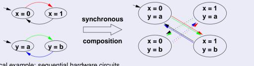
• Typical example: sequential hardware circuits.
