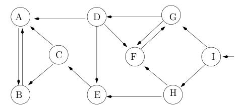
Given the graph in the figure, draw the sequence of arcs explored by a breadth-first search (BFS) starting from the node I. (Notation: use e.g., "AB" to denote the arc " $A \longrightarrow B$ ".) [Solution:
