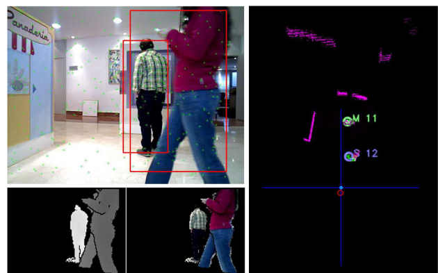
Fig. 9 Snapshot of the execution of people tracking algorithm. Bottom left the depth and RGB maps corresponding to independently moving people. Right a top view of the local environment map showing the motion hypotheses for two people. Top left the bounding boxes of the identified moving persons
