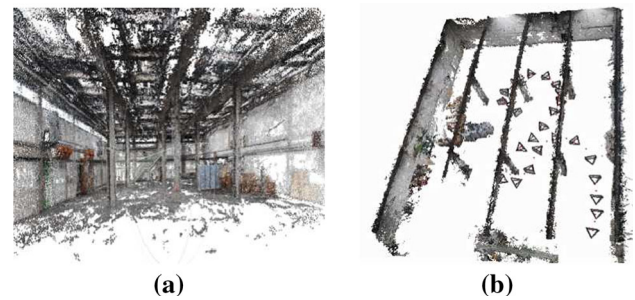
Fig. 5 3D point cloud data derived from our “Structure from Motion”-Workflow
