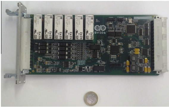
Fig. 6. The board SV106 implementing one of the safety channels of the SAFE-MOD unit.
