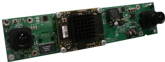
Fig. 7. Prototype board for the proposed system, with a baseline of 15 cm.
