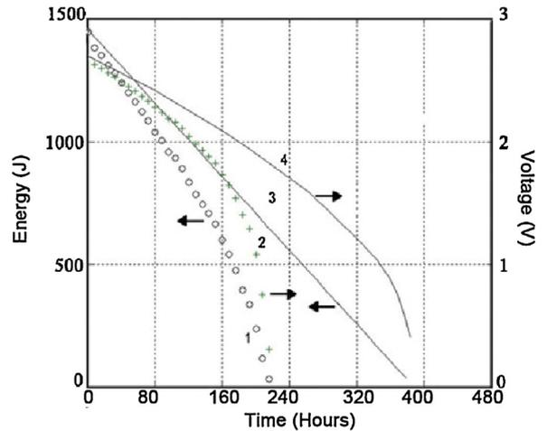
Fig. 10. Theoretical (solid curve) and experimental dependences (dots curve) for the supercapacitor energy (curve '1' and '3') and voltage (curve '2' and '4') during wireless sensor gas node operation.
