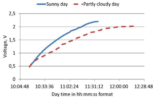
Fig. 8. Super capacitor charging through the solar panel.
