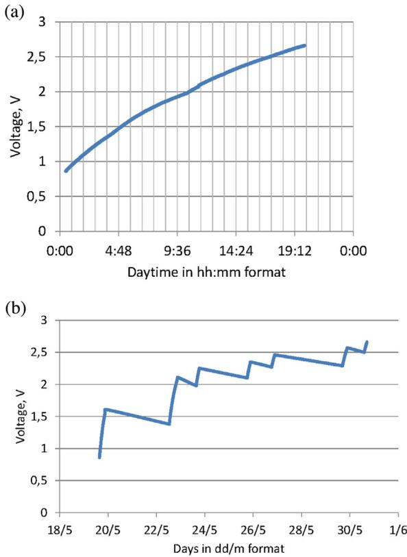
Fig. 7. Charging of the super capacitor from the wind generator: (a) continuous charging at wind speed of 4 m/s, (b) charging from the wind depending on its availability.
