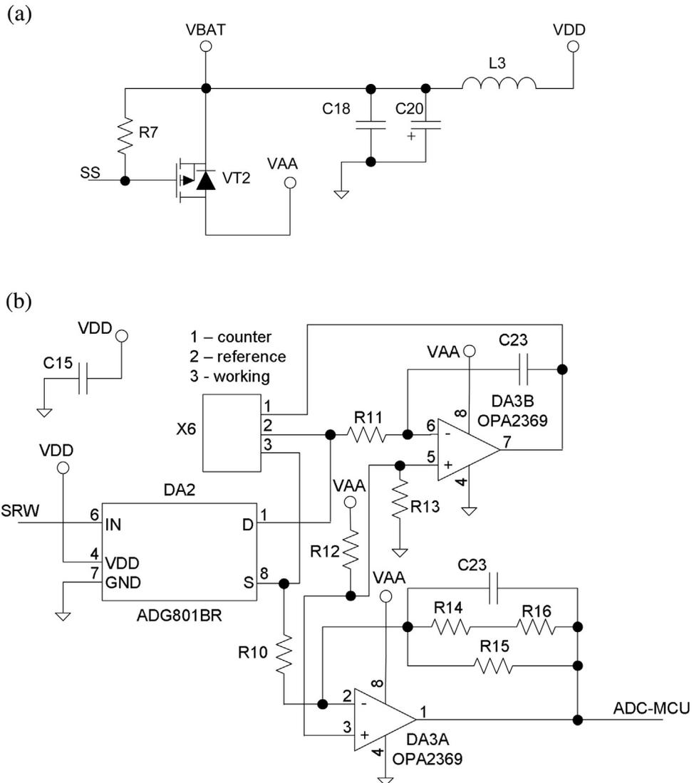
Fig. 2. Analog sensing circuit: (a) sensing circuit switch and (b) sensing circuit where X6 is the CO sensor.
