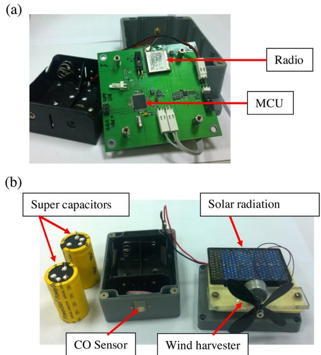
Fig. 4. Prototype of the wireless sensor node for CO monitoring: (a) a board with the MCU and wireless transceiver, (b) harvesters, super capacitors and CO sensor in packaging.
