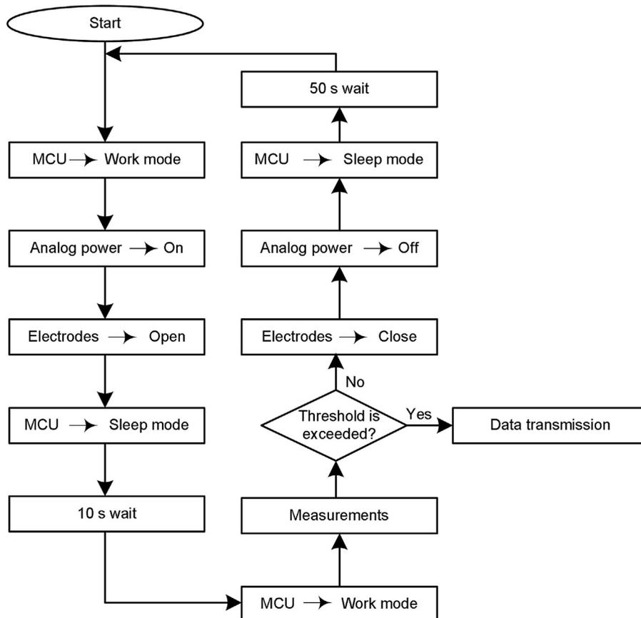
Fig. 6. Algorithm showing how the sensor node conducts gas measurement.
