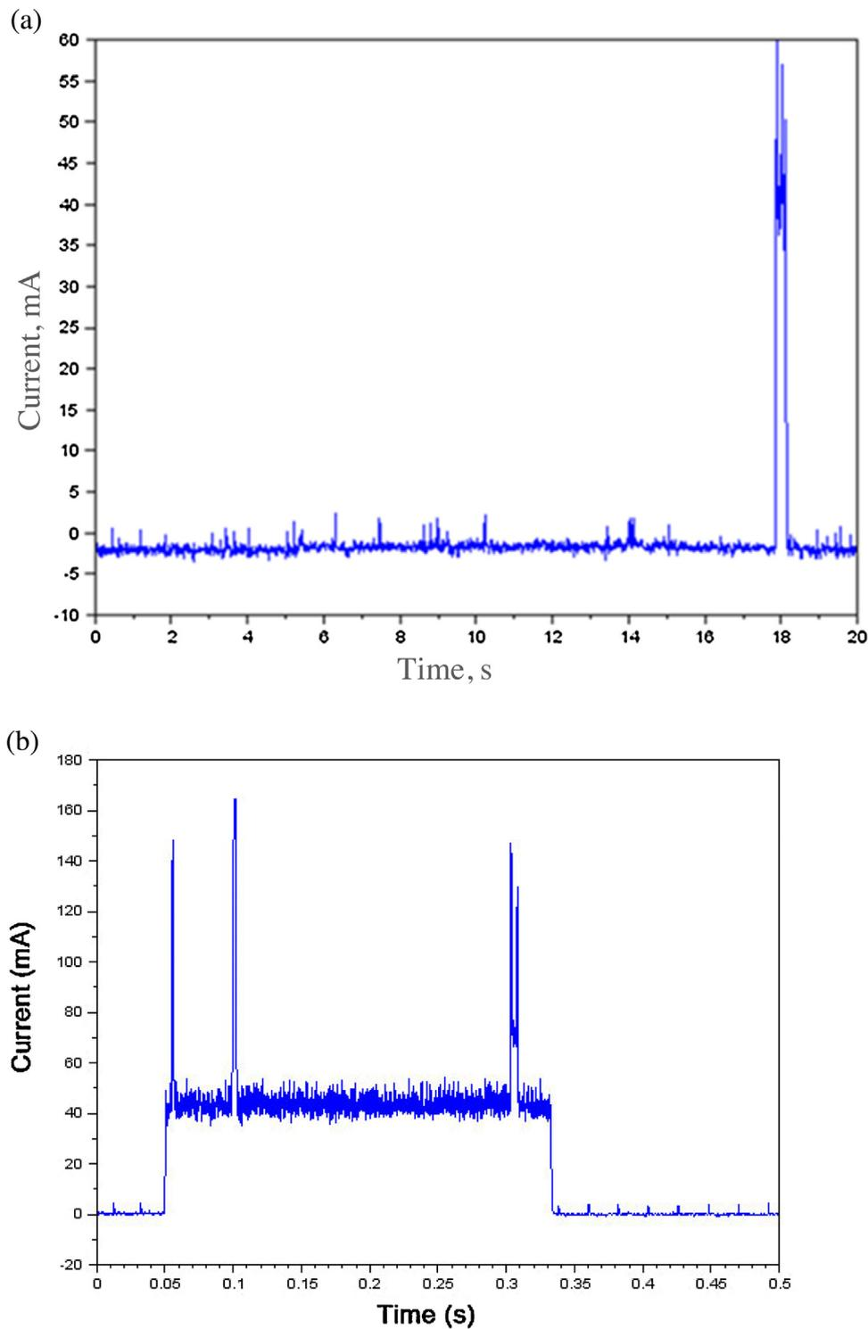
Fig. 11. Current consumption of sensor node: (a) in sensing mode and (b) average current consumption (sensing and data transmission) is 43.49 mA within 0.28 s.
