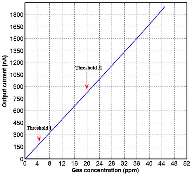
Fig. 5. Curve showing sensor response (output current) w.r.t. CO concentration.
