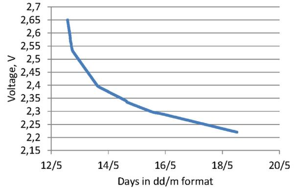
Fig. 9. Super capacitor self-discharge within 6 days.
