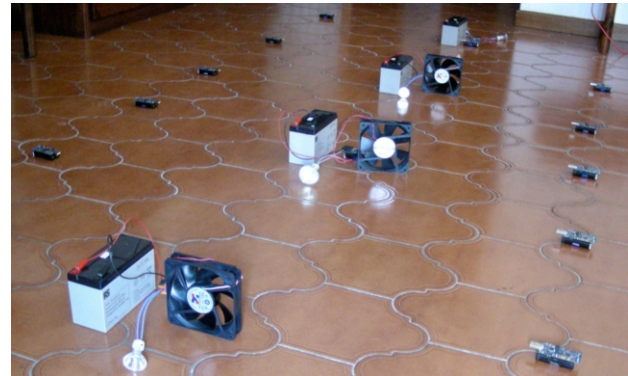
Fig. 5: Overall setup and nodes controlling fans and lights.
