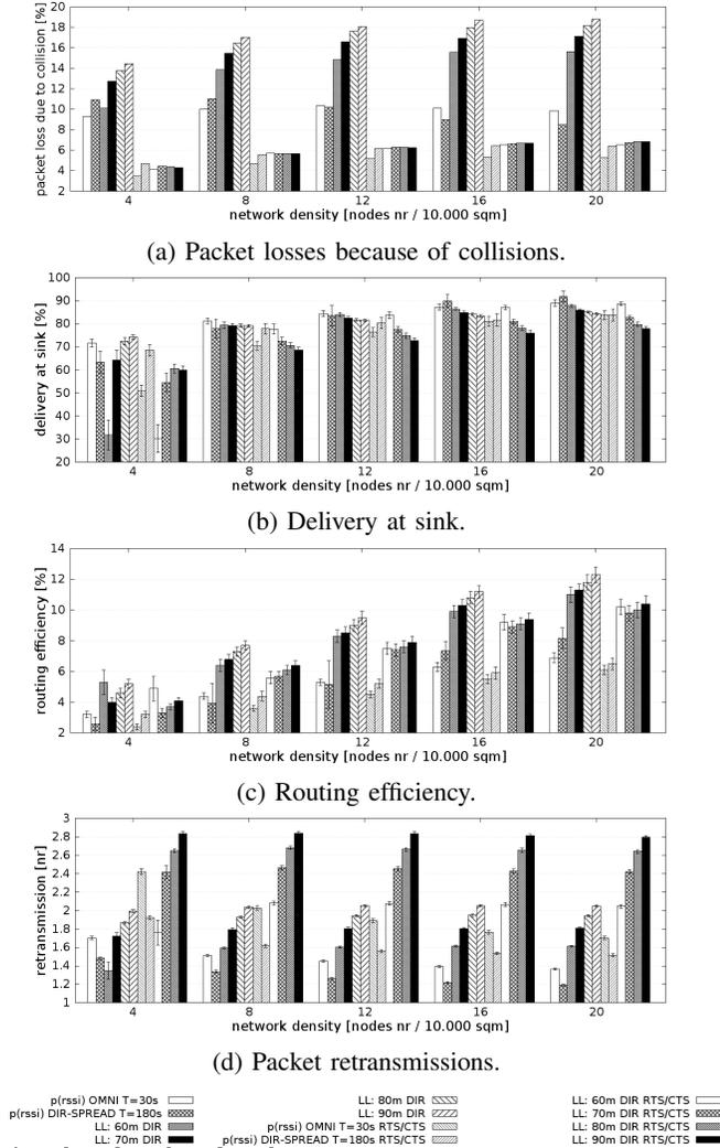
Figure 10: Using RTS/CTS to cope with hidden terminals.
