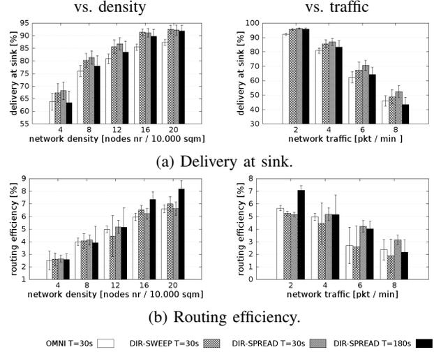
Figure 4: Impact of link probing.
