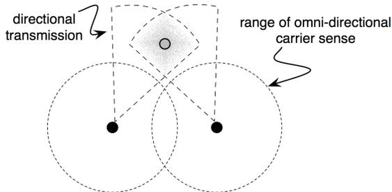
Figure 8: Two nearby transmitters address the same receiver in a directional manner; due to omni-directional CSMA, carrier sense fails and packets collide at the receiver.
