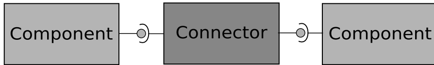
(b) A connector component as it is actually bound to the components it is meant to connect. The connector interfaces and receptacles mimic those of the components bound.
