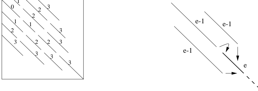
Figure 11: On the left, the O(k^2) algorithm to compute the edit distance. On the right, the way to compute the strokes in diagonal transition algorithms. The solid bold line is guaranteed to be part of the new stroke of e errors, while the dashed part continues as long as both strings match.
