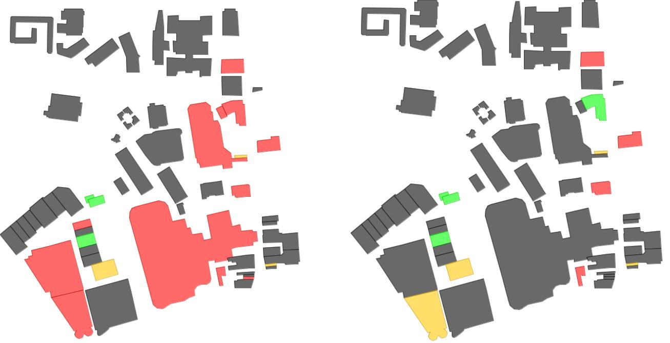
Figure 4. Object Matching Results without Validation (left) vs. Results with Validation (right): TP: Black; FP: Red; TN: Yellow; FN: Green.
