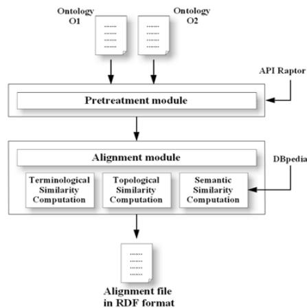
**Fig. 1.** Sketch of architecture for LDOA method
