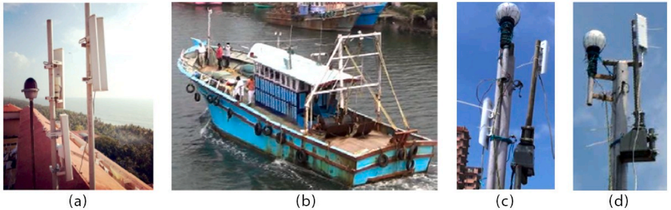
Fig. 7. Testbed setup for the network architecture: (a) Base Station setup at the shore, (b) Fishing vessel as a node, (c) SuperNode acts as mobile BS and ABE, (d) Adaptive Node or ABE.
