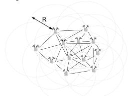
Many links  $\rightarrow$  no leaf nodes  $\rightarrow$  tolerant to one failure.
