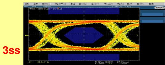
Eye Pattern with Mask: 1000B - SX/LX (1.25Gb/s) at location 3 with single mode Fibre
