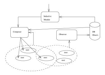
Figure 3: The System for Implicit Culture Support. The basic architecture for the System for Implicit Culture Support consists of the following three basic components: the *observer* that stores in a database (DB) the information about the executed user actions in order to make it available for other components; the *inductive module* that analyzes the executed actions in order to discover patterns of user behaviors; the *composer* that produces the links to suggest the user
