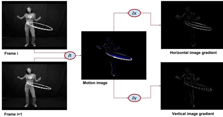
Fig. 2: Visualization of the process for capturing the motion information for the HMG descriptor. We initially perform a fast temporal derivation over each two consecutive frames, which provides us the motion image. Then we compute the horizontal and vertical gradients for the resulted motion image. The pixels depicted in blue color represent the negative values after temporal derivation.
