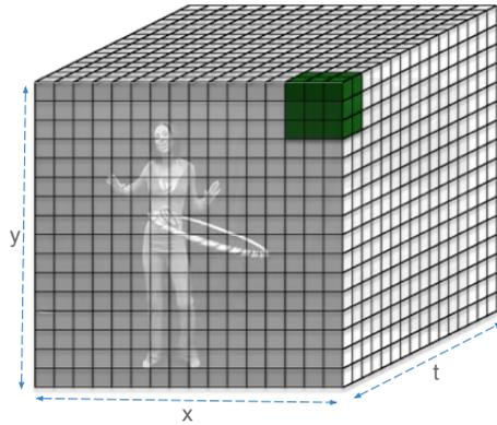
Fig. 3: The process of dividing the video in blocks and volumes. The part depicted in green represents an illustration of a volume created from 3 by 3 by 2 blocks.
