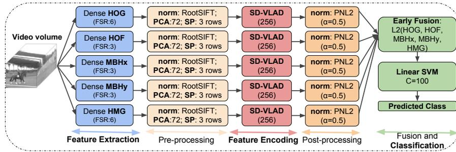
Fig. 7: The pipeline for real-time video classification. This framework can process the video at a speed of 39 frames/second and yields an accuracy of 0.845 on UCF50 dataset, 0.767 on UCF101 and 0.470 on HMDB51.
