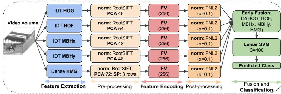
Fig. 8: The pipeline for accurate video classification. This framework yields an accuracy of 0.930 on UCF50 dataset, 0.881 on UCF101 and 0.610 on HMDB51, but can process only 3 frames/second.
