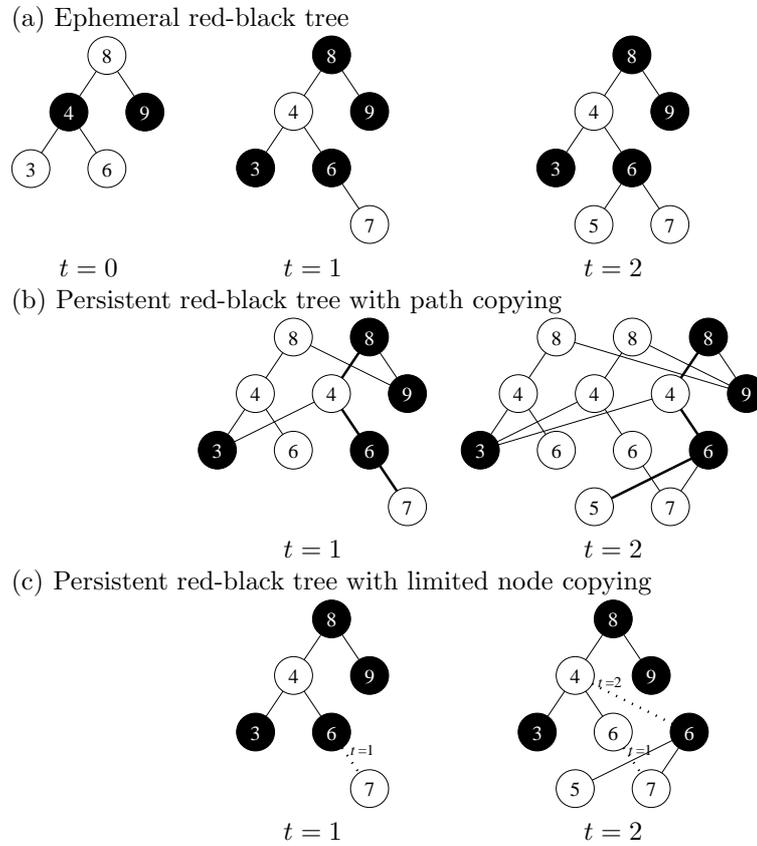
Figure 3: How to obtain a partially persistent red-black tree from an ephemeral one (top), containing indices 3,4,6,8,9 at  $t=0$ , with subsequent insertion of 7 and 5. Path copying (middle), with thick lines marking the copied part. Limited node copying (bottom) with dashed lines denoting the “extra” pointers with time stamp.
