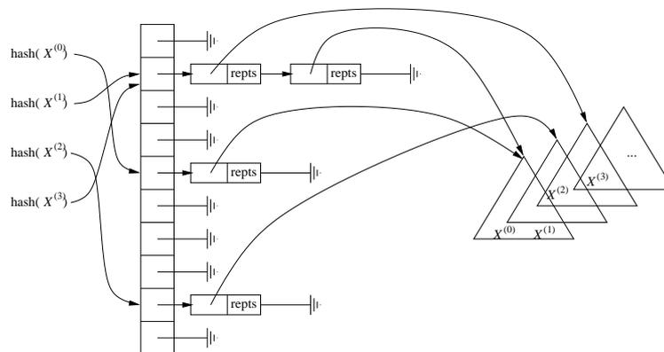
Figure 4: Open hashing scheme with persistent sets: a pointer to the appropriate root for configuration  $X^{(t)}$  in the persistent search tree is stored in a linked list at a “bucket”. Items on the list contain satellite data. The index of the bucket array is calculated from the configuration through a hashing function.
