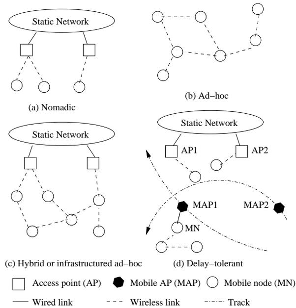
Figure 1: Wireless network architectures
