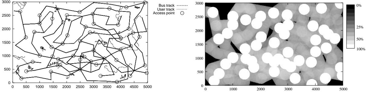
Figure 4: (Left) Bus lines and user tracks. (Right) corresponding time of coverage during the simulation. Note that the greyscale is not linear.
