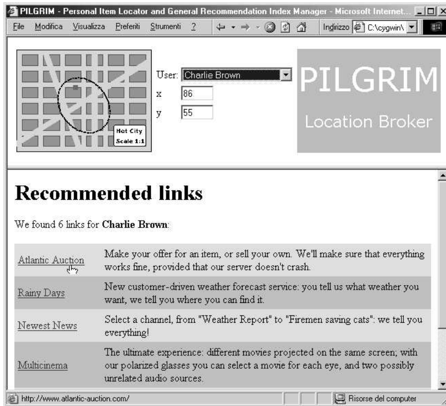
Fig. 4. Screenshot of the experimental PILGRIM system. User identity, location and map are shown on the top frame; the bottom frame contains an item recommendation list; the ellipse in the map represents the inertial ellipsoid of the link under the mouse pointer.
