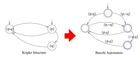
⇒ Substantially, add one initial state, move labels from states to incoming edges, set all states as accepting states
