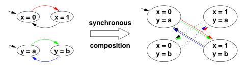
• Typical example: sequential hardware circuits.
