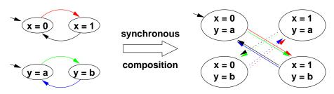
• Typical example: sequential hardware circuits.
