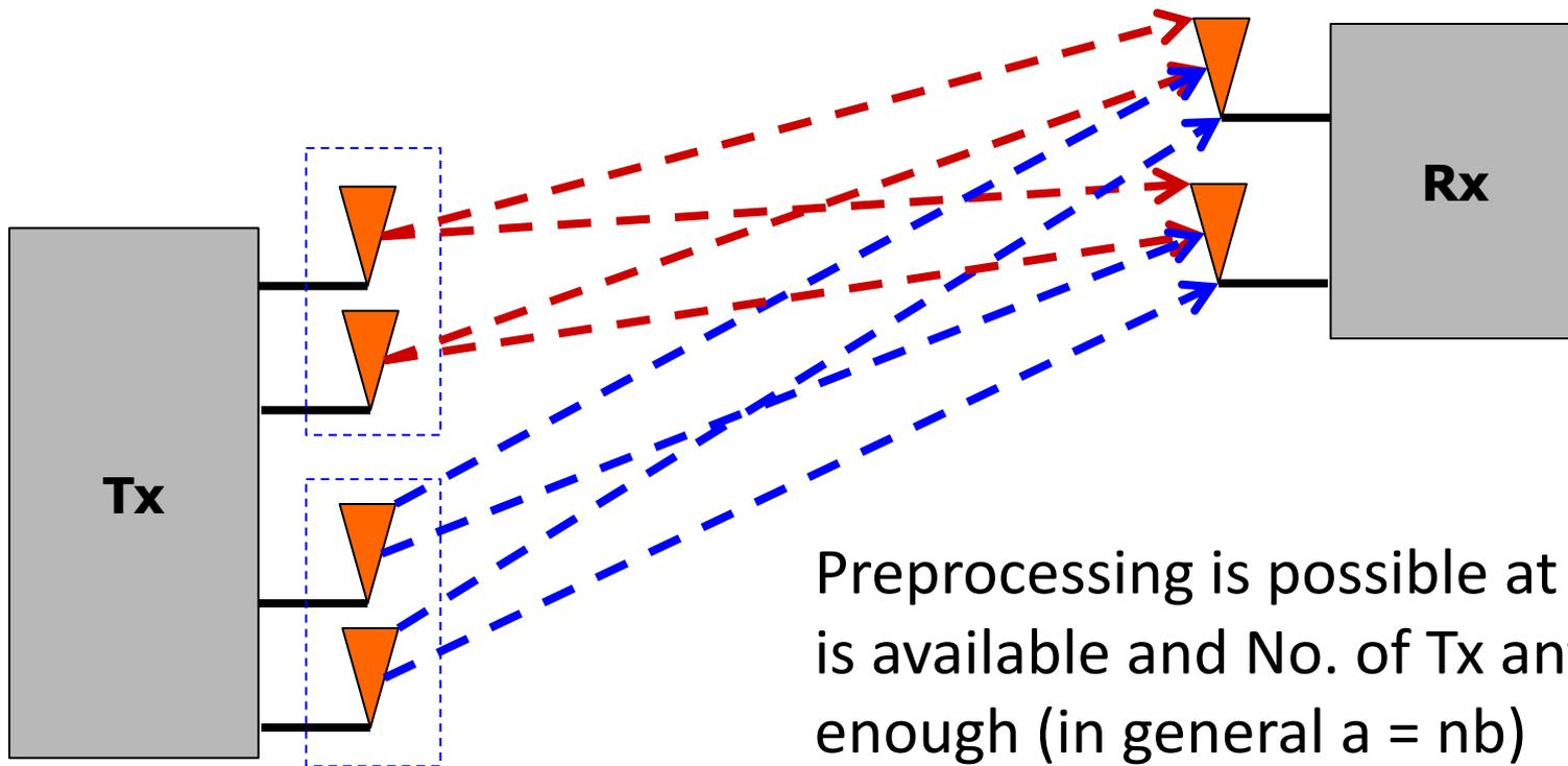
Preprocessing is possible at Tx if CSI is available and No. of Tx antennas is enough (in general  $a = nb$ )
