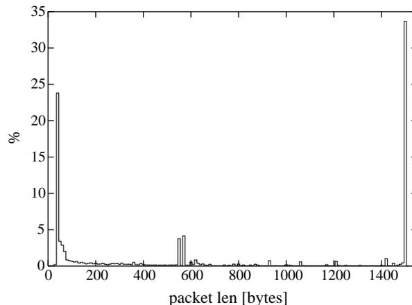
Fig. 7. Packet length distribution used in simulations.
