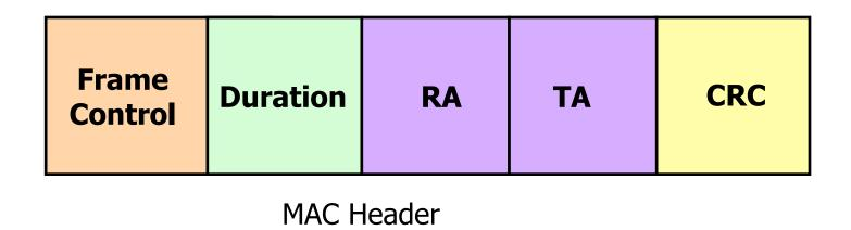
**Duration** (in μs): Time required to transmit next (data) frame + CTS + ACK + 3 SIFs
