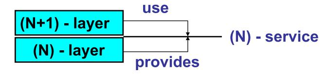
In TCP/IP this are the "socket" between application layer protocols and TCP/UDP
