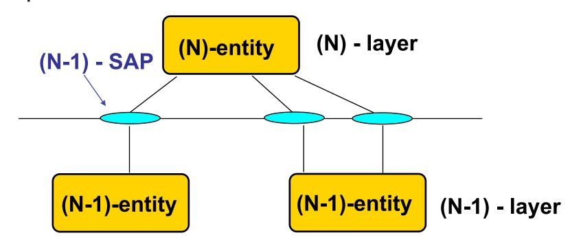
In Internet we have many different names for SAPs, from sockets to buffer to simply c-functions non formally named (e.g., the "ethernet" interface of Linux kernels
