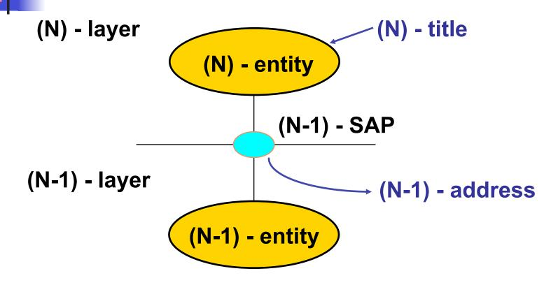
In TCP/IP addresses are named "port", "protocol", depending on the layers
