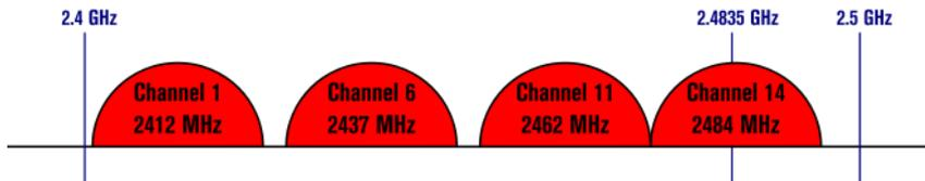
802.11g/n (OFDM) 20 MHz ch. width - 16.25 MHz used by sub-carriers
