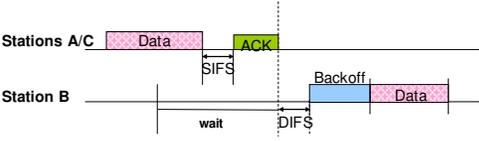
The diagram illustrates the Basic DCF protocol. Station A/C sends a Data frame (pink box). Station B receives it and sends an ACK (green box). Station A/C receives the ACK and sends a SIFS (Short Inter Frame Space) interval. Station B then enters a 'wait' period, followed by a 'Backoff' period (blue box), and finally sends its own Data frame (pink box). A DIFS (Distributed Inter Frame Space) interval is shown between the end of Station A/C's ACK and the start of Station B's Data frame.
