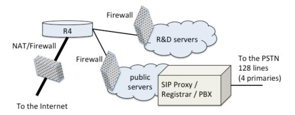
The VoIP services can interconnect the company system to other VoIP systems through the standard Internet access, but they must be interconnected to the traditional PSTN for global service. 128 lines of interconnection can be a good dimension for this part:
