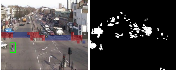
Figure 3. (Left) Anomaly. Pedestrian detected outside associated semantic map. (Right) corresponding Foreground mask.
