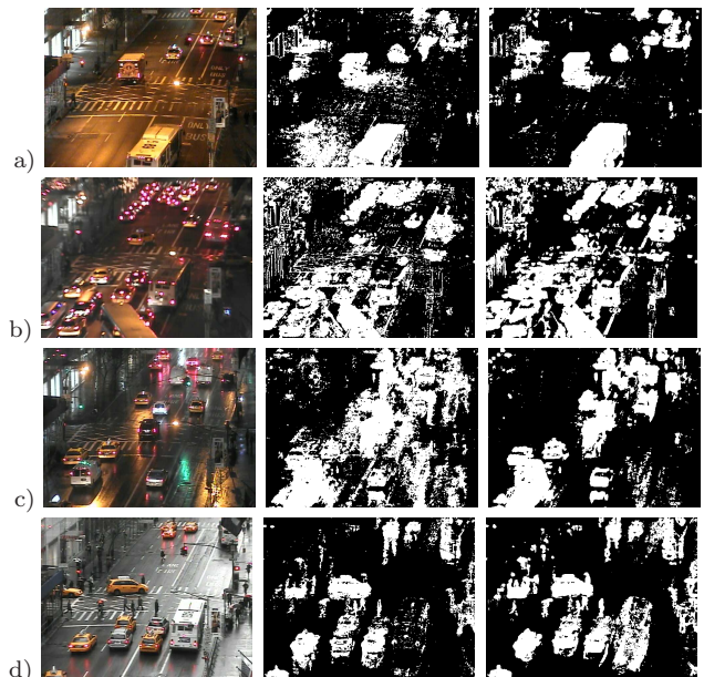
Figure 5: Performance on foreground detection w.r.t. different challenges: (a) sudden light changes, (b) sudden image blurring (camera defocus), (c) night lighting with rain, (d) stationary foreground. (Left) original frame, (center) [32], (right) our method.
