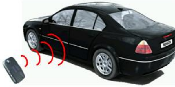
Figure 34: Automotive localisation system based on UWB
