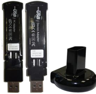
Figure 29: WISAIR Wireless USB adapter set (PC adapter, device adapter, table adapter)
