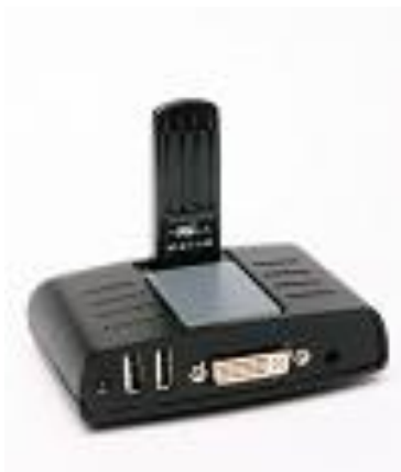
Figure 28: WISAIR wireless DisplayDock device side (PC device adapter)
