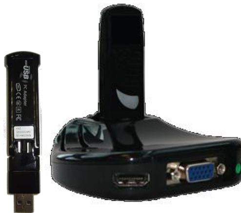
Figure 26: WISAIR Wireless USB adapter set (PC adapter, AV adapter with device)
