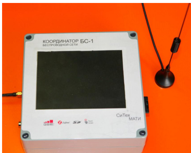
Fig. 4. The implementation of the network coordinator, based on the LPC2478 microprocessor, in casing. The LCD display on top is used to show the operational status of the network.
