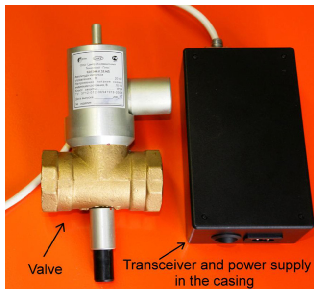
Fig. 5. Wireless actuator contains the valve for gas emission source control and the casing with the ZigBee transceiver and power supply inside.
