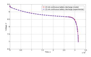
Figure 6. Battery discharging with continuous 23 mA current
