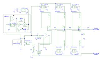
Figure 5. Spice model of a NiMH battery
