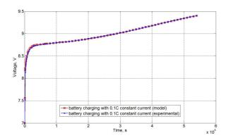
Figure 7. Continuous battery charging (0.1C)
