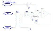
Figure 3. Controllable resistor
