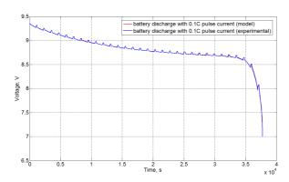
Figure 8. Pulse battery discharging (0.1C)
