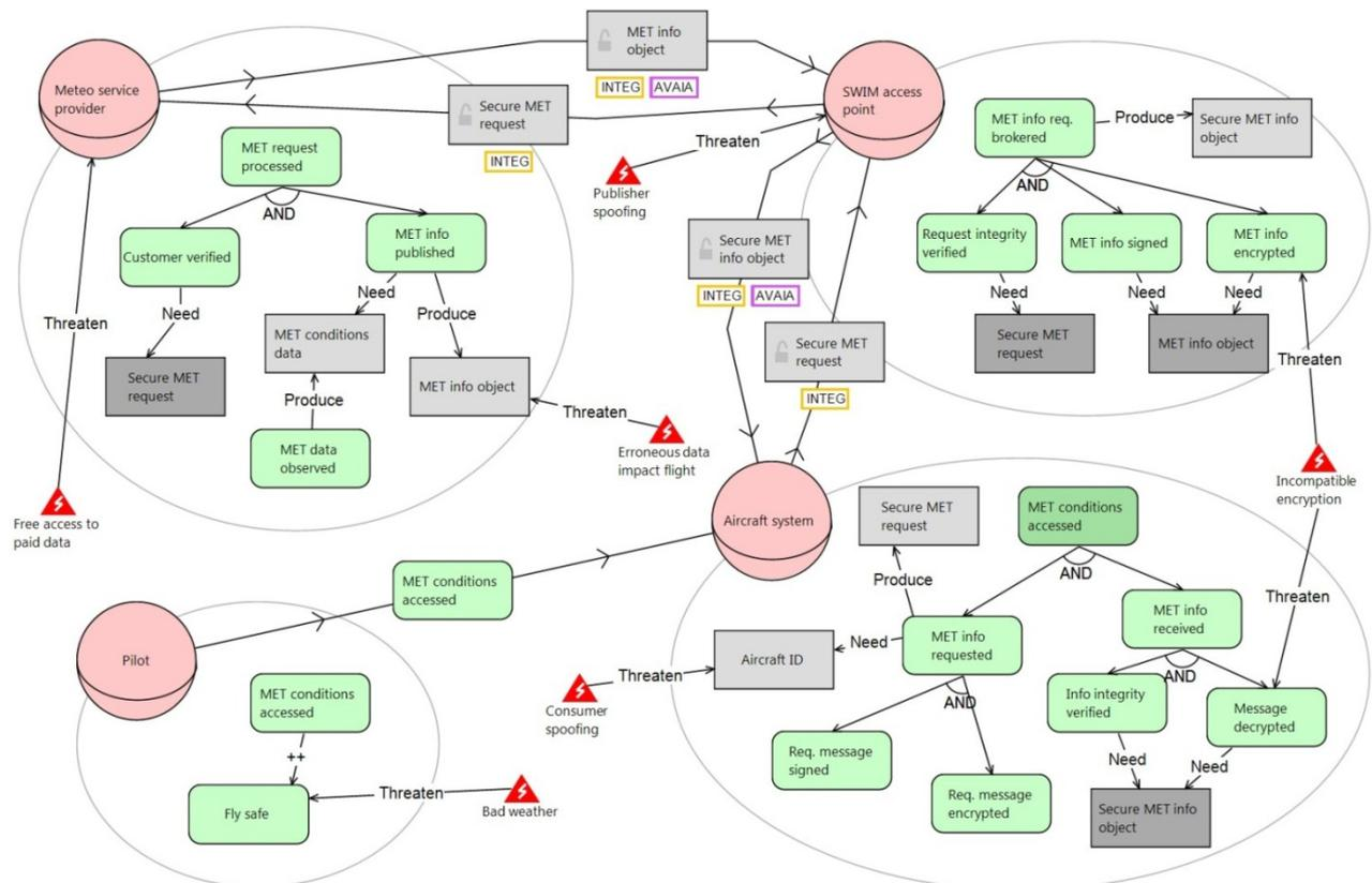
Figure 1. An STS-ml model for the ATM scenario with events and *threaten* relationships
