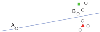
Figure 5.1: An illustration of when uncertainty sampling can be a poor strategy. Shaded polygons represent labeled instances in \mathcal{L} , and circles represent unlabeled instances in \mathcal{U} . Since A is on the decision boundary, it would be queried as the most uncertain. However, B would probably provide more information about the input distribution as a whole.
