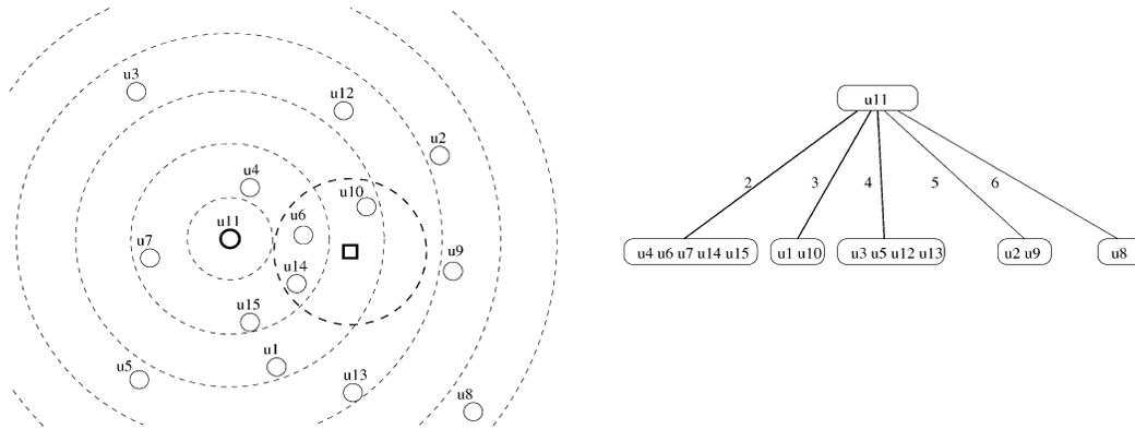
**Fig. 2.** On the left, the division of the space obtained when  $u_{11}$  is taken as a pivot. On the right, the first level of a BKT with  $u_{11}$  as root. We also show a query  $q$  and the branches that it has to traverse. We have discretized the distances so they return integer values.
