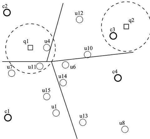
**Fig. 13.** A compact partition using four centers and two query balls intersecting some classes. Note that the class of  $c_3$  could be excluded from consideration for  $q_1$  by using the covering radius criterion but not the hyperplane criterion, whereas the opposite happens to discard  $c_4$  for  $q_2$ .
