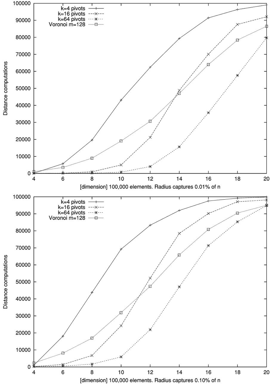
**Fig. 19.** Distance evaluations for increasing dimension. We compare the compact partitioning algorithm of Figure 18 using 128 centers per level against the filtration using  $k$  pivots for  $k = 4, 16, 64$ . On top the search radius captures 0.01% of the set, on the bottom 0.1%.
