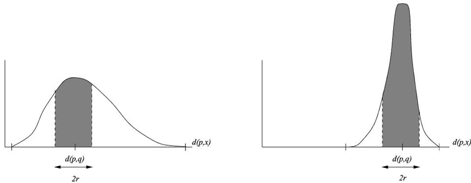
**Fig. 14.** A low-dimensional (left) and high-dimensional (right) histogram of distances, showing that on high dimensions virtually all the elements become candidates for exhaustive evaluation. Moreover, we should use a larger  $r$  in the second plot in order to retrieve some elements.
