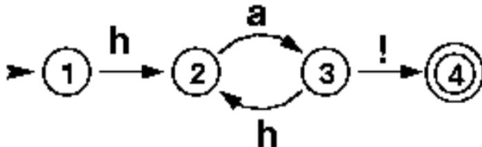
The nodes of the graph are the states of the generator. We have numbered them, so that it is easier to talk about them. The **arcs** of the graph are the transitions, and the **labels** of the arcs are the symbols that the machine emits. A double circle indicates that this state is a final state and the one with the black triangle is the start.
